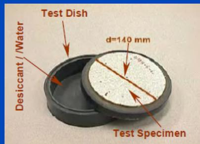
Example specimen and test apparatus that is placed into an environmental chamber to measure WVT.
