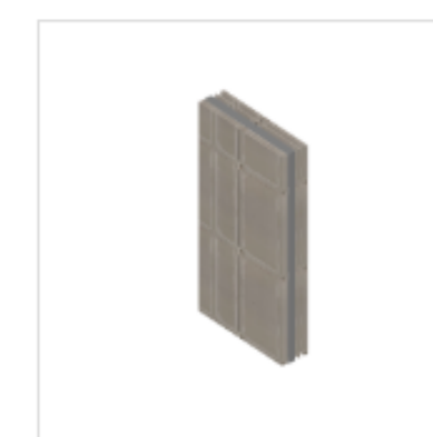
3-5/8" METAL STUDS WITH 3 LAYER / 3 LAYER GYPSUM BOARD
