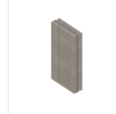
3-5/8" METAL STUDS WITH 4 LAYER / 4 LAYER GYPSUM BOARD
