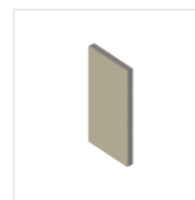
3-5/8" METAL STUDS W/ 1 LAYER / 1 LAYER GYP. BD.
